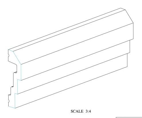
Density: ---- kg /dm³ Volume: 0,783 dm³ /m Weight: ---- kg /m Paint surf: 10,875 dm² /m
